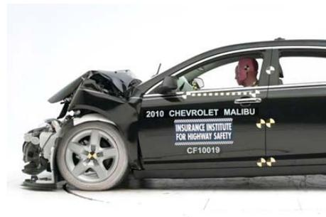
This is a car after a 35 mph full-width crash into a Wabash trailer with a strong guard. The occupant compartment is intact.
