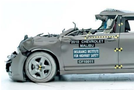
This is how a car looks after a 35 mph full-width crash into the rear of a Hyundai trailer with a weak Under-ride guard.
